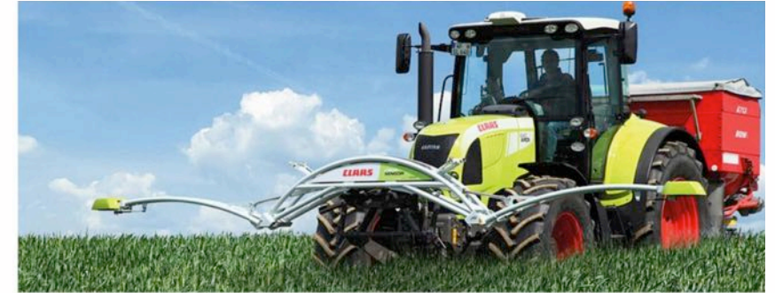
Abbildung 6: Crop Sensor (© Claas Agrosystems)
